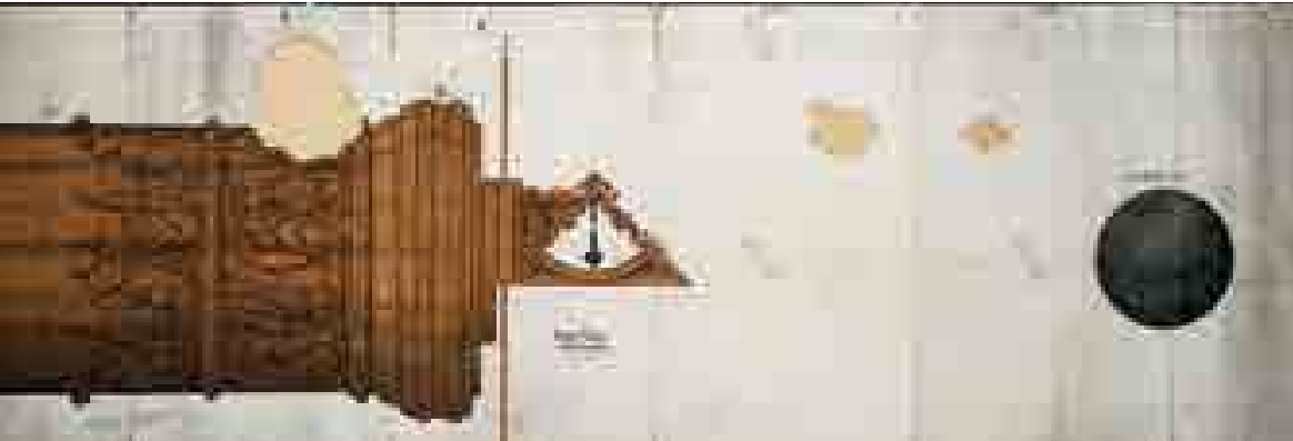
Depiction of the muzzle of a piece of artillery with aiming device and projectile, Paulus Puchner, 1577
